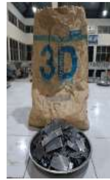
Gambar 5. Steel Fibre tipe hooked-end
