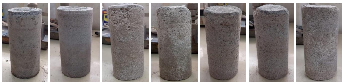
Gambar 8. Benda Uji (a) Normal (b) ASP 0% + SK 10% (c) ASP 5% + SK 10% (d) ASP 10% + SK 10% (e) ASP 15% + SK 10% (f) ASP 20% + SK 10% (g) ASP 25% + SK 10%
