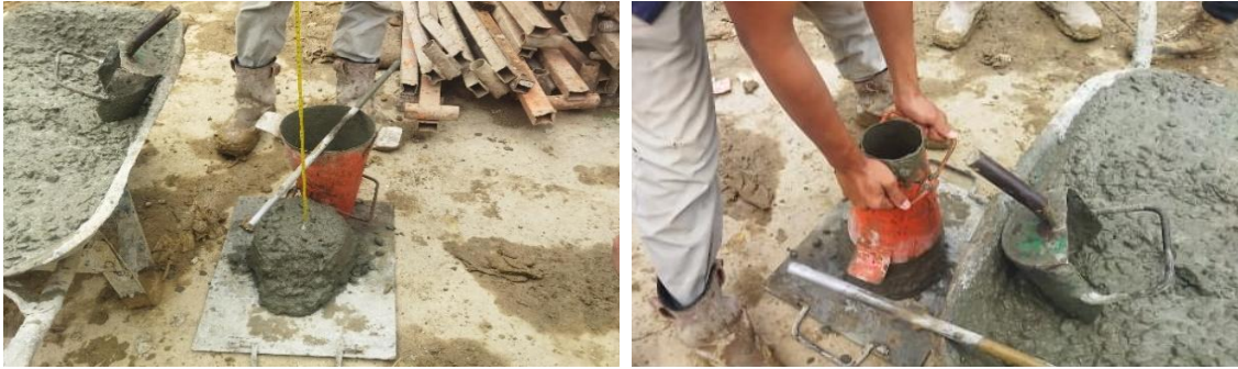
Gambar 1. Proses pengujian Slump Beton
