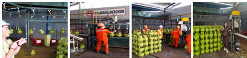
Gambar 2. Proses retester , repair , dan repaint plant tabung LPG 3kg
