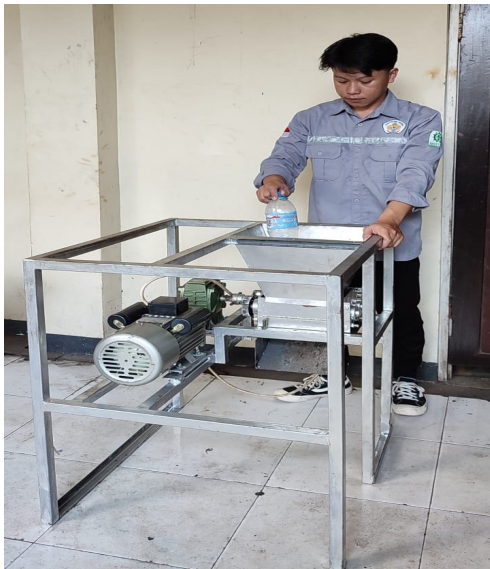
Gambar 4. mesin pencacah sampah plastik Tipe Shredded Claw Blade Double Shaft
